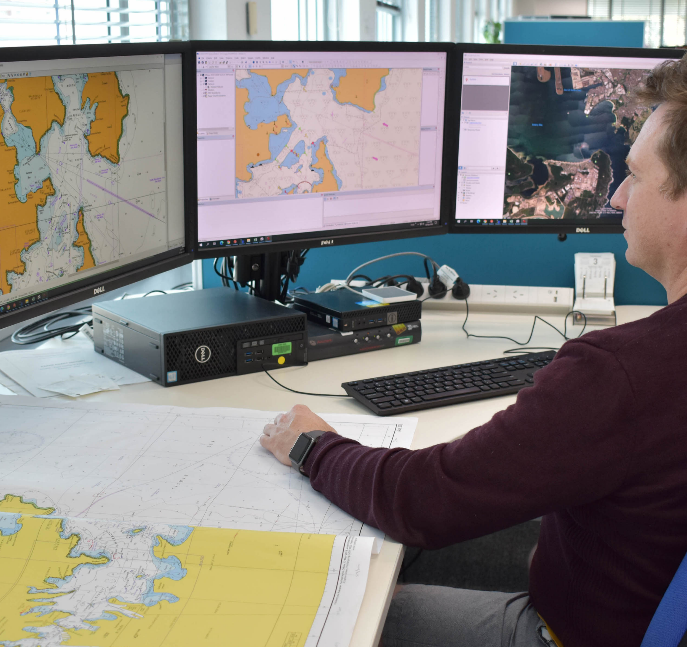
At the Australian Hydrographic Office, a nautical cartographer works on some of Australia's 1342 official paper and electronic nautical charts, combining historic data with contemporary imagery and satellite derived bathymetry. Source: Australian Hydrographic Office
