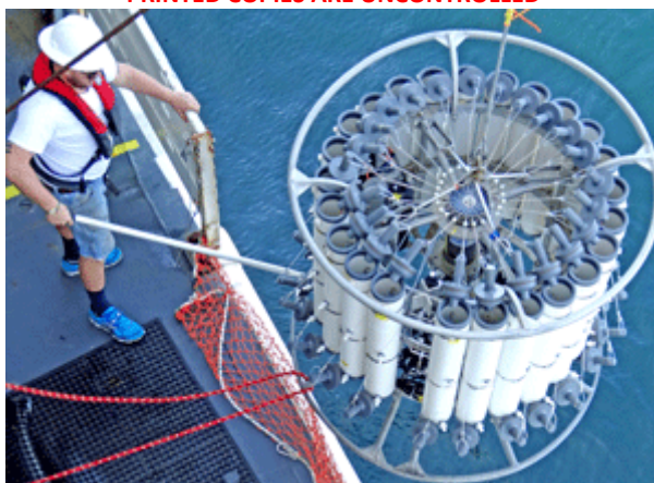
Figure 9 – CTD probe surrounded by a rosette of Niskin water sample bottles
